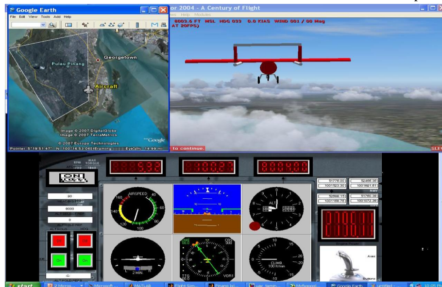
Figure 9: Nonlinear, non real time simulation of waypoints following for UAV
