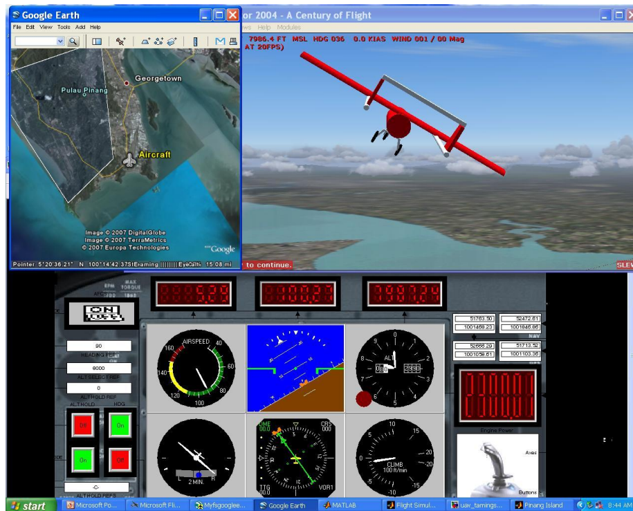
Figure 10: Nonlinear, non real time simulation of heading hold/select for UAV
