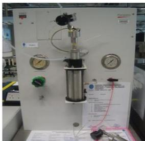
**Fig. 4:** The Poroperm device
