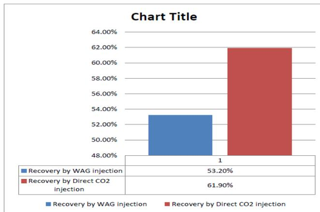
**Fig. 5:** Recovery profile by WAG and direct CO<sub>2</sub> injection alone.
