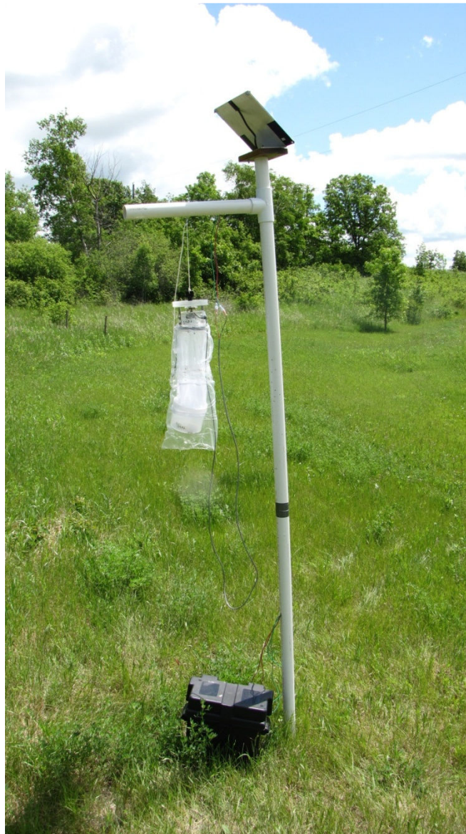
Figure 1. The solar-powered CDC light trap system. The bag on the trap prevents rain and dew from damaging mosquitoes in the collection bag attached to the trap.
