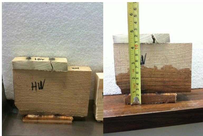
Figure 3.(a) Specimen with initial water level of 1 cm (left) and (b) water penetration height measurement (right)
