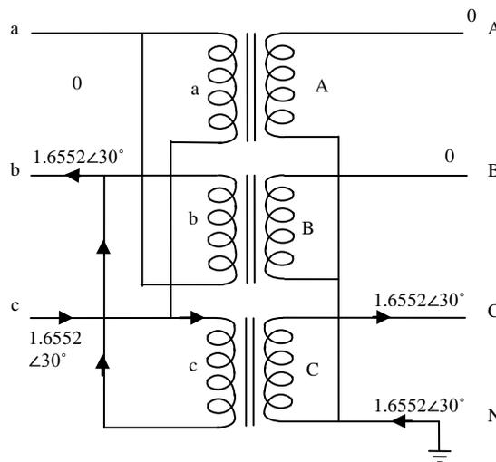
**Figure 4c:** Transformer currents for a line-to-ground fault in phase *c*
