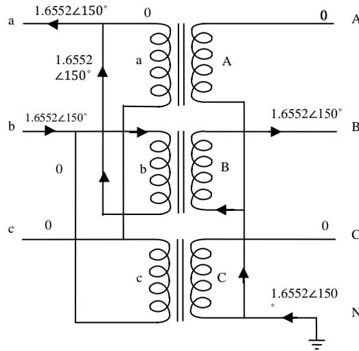
**Figure 4b:** Transformer currents for a line-to-ground fault in phase *b*.
