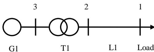
**Figure 2:** Sample Three Bus Bar System
