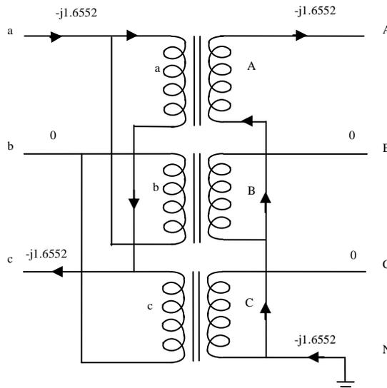
**Figure 4a:** Transformer currents for a line-to-ground fault in phase *a*.
