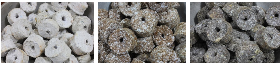
Figure 4: Types of briquettes produced using biomass wastes, from left to right: a) paper, b) paper + sawdust, and c) paper + sawdust + CRH.
