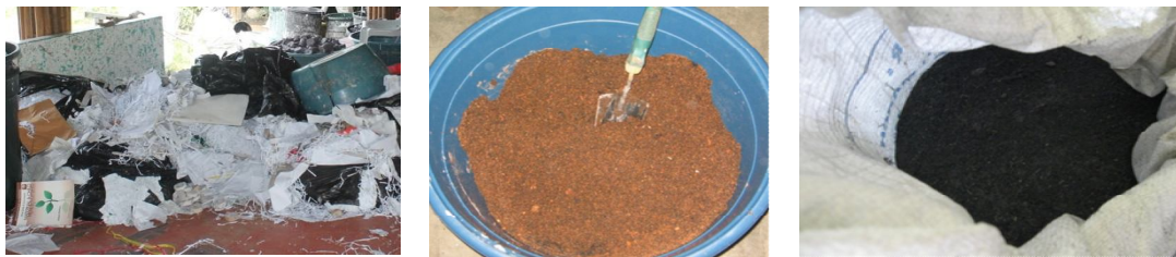
Figure 2: The materials used in briquette production, namely, from left to right: waste paper, sawdust and carbonized rice husk.
