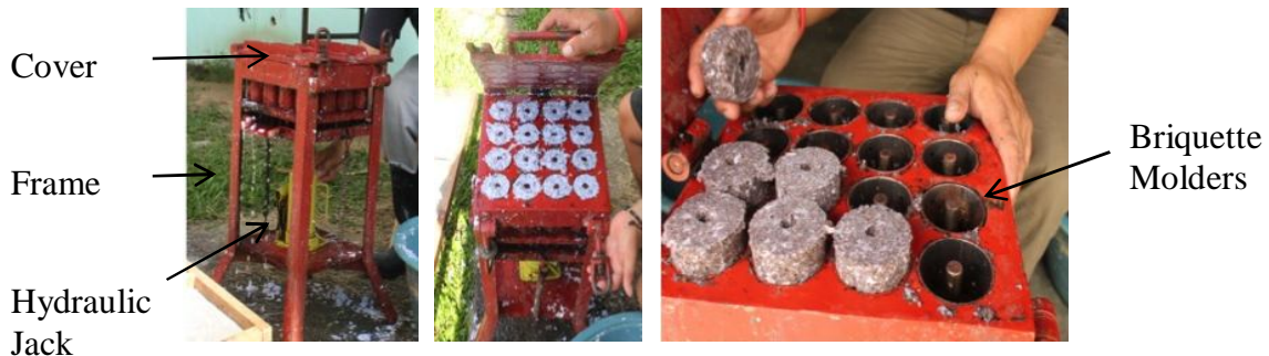
Figure 1: The hydraulic jack-driven briquetting machine utilized in the biomass briquette production test.
