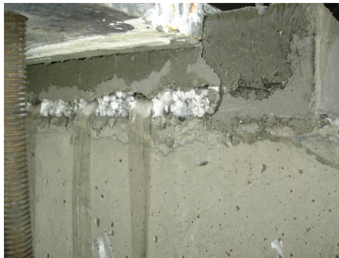
Fig. 4. Foam plates in the pure torsion test
