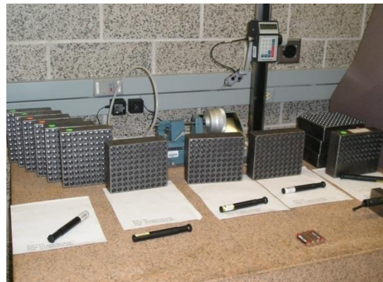
Figure 2: Drilled Work Pieces
