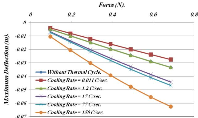
Fig.(4): Variation of Max. Deflection due to Applied Force for Different Cooling Rates Using Non-Linear Analyzing by ANSYS Software.
