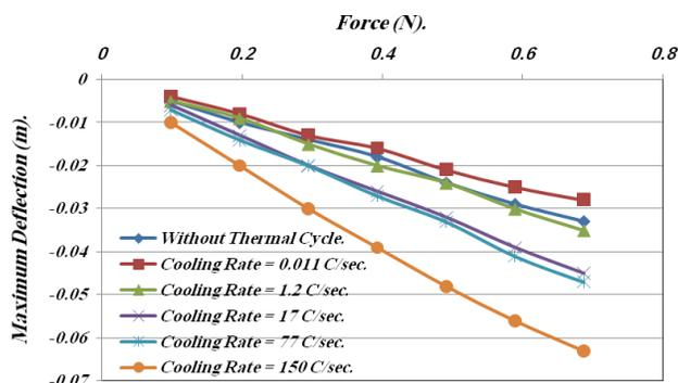
Fig.(7): Experimental Results of Variation of Max. Deflection due to Applied Force for Different Cooling Rates.
