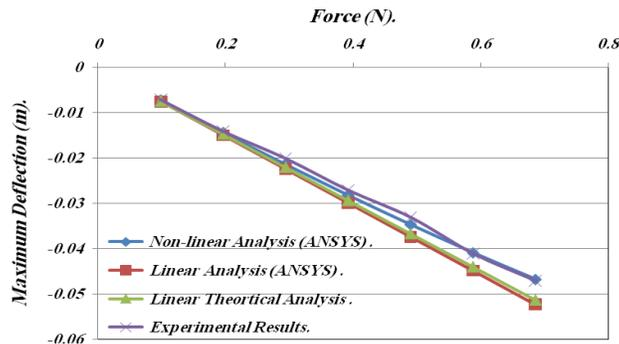
Fig.(12). Comparison Between Different Techniques to calculate Max. Deflection due to Applied Force for Cooling Rates= 77 C°/Sec.
