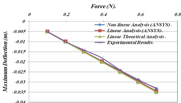
Fig.(8). Comparison Between Different Techniques to calculate Max. Deflection due to Applied Force for Beam Without Thermal Cycle.
