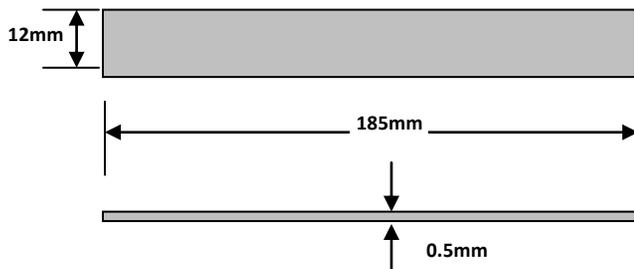
Fig.2.The dimensions of stainless steel sample.
