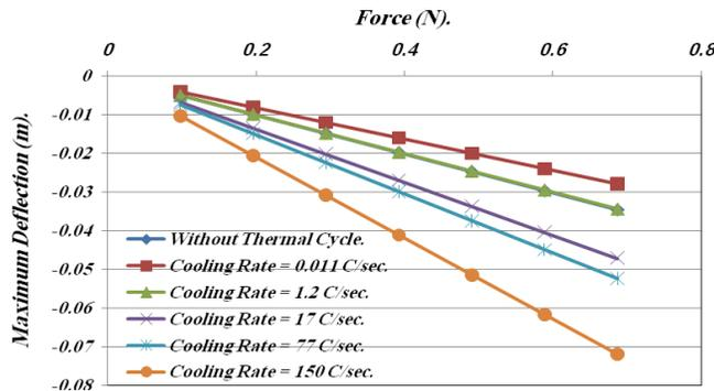
Fig.(5): Variation of Max. Deflection due to Applied Force for Different Cooling Rates Using Linear Analyzing by ANSYS Software.
