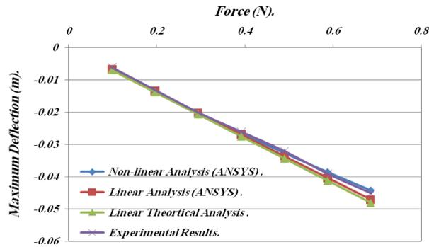
Fig.(11). Comparison Between Different Techniques to calculate Max. Deflection due to Applied Force for Cooling Rates= 17 C°/Sec.
