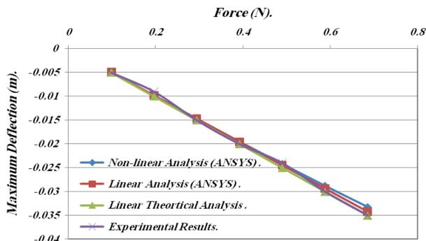
Fig.(10). Comparison Between Different Techniques to calculate Max. Deflection due to Applied Force for Cooling Rates= 1.2 C<sup>o</sup>/Sec.
