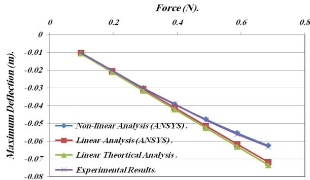
Fig.(13). Comparison Between Different Techniques to calculate Max. Deflection due to Applied Force for Cooling Rates= 150C°/Sec.
