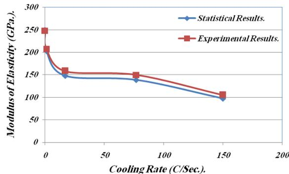
Fig.(14):Comparison Between Experimental and Statistical Results of Modulus of Elasticity When the Cooling Rate Changes.
