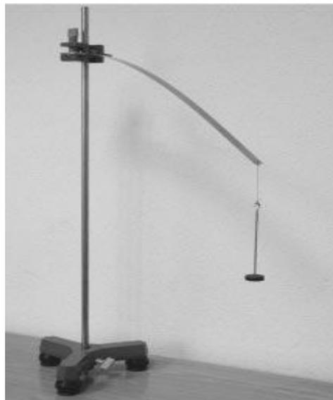
Fig. 3. Photograph of a cantilever beam loaded with an external vertical concentrated load at the free end.
