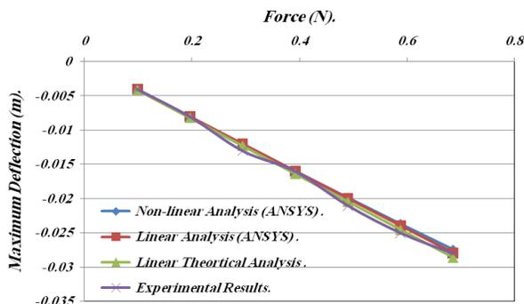
Fig.(9). Comparison Between Different Techniques to calculate Max. Deflection due to Applied Force for Cooling Rates= 0.011 C<sup>o</sup>/Sec.
