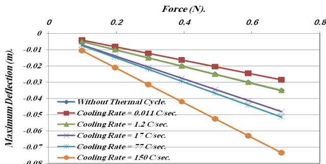
Fig.(6): Variation of Max. Deflection due to Applied Force for Different Cooling Rates Using Linear Analyzing.
