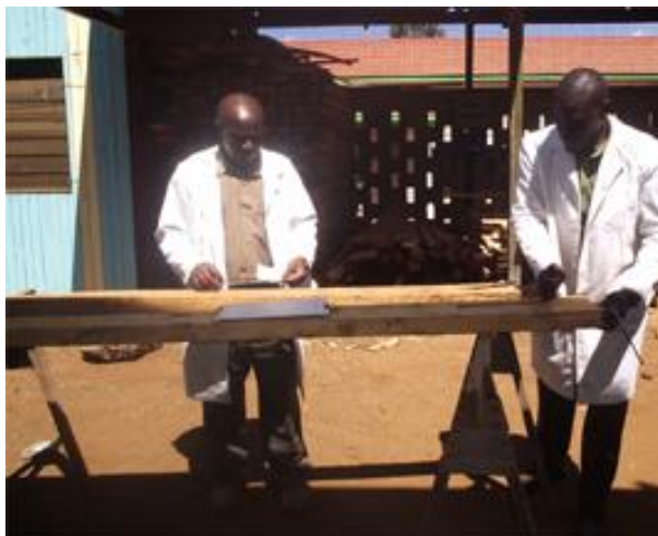
Figure 2. Grading sawn timber into SS, GS and Reject grades
