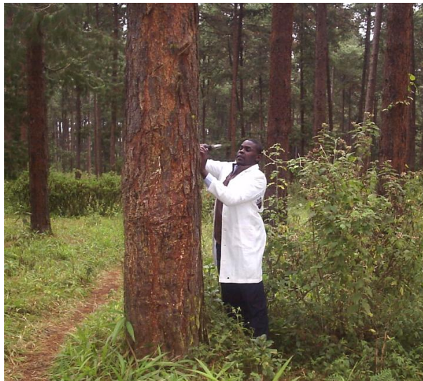
Figure 1. Determination of spiral grain angle on standing tree in Muguga
