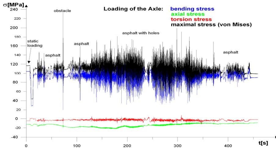
Fig. 4 The stresses in the section of the axle during full loading in various service condition
