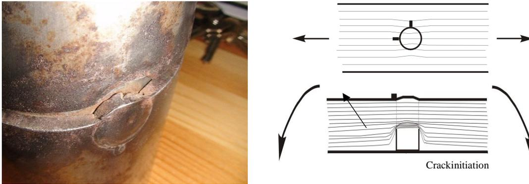
**Fig. 2** Fracture surface detail and scheme of force-flow
