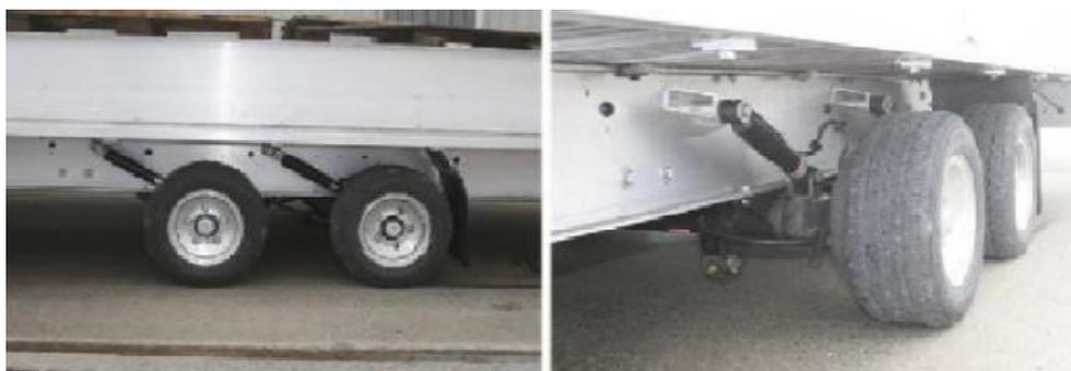
**Fig. 1** Height-adjustable chassis the special lorry FGS
