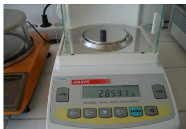
Figure 6: Electronic Scale with a Precision of 1/10000
