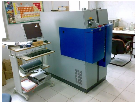
Figure1: Spektrolab Instrument With19 Elements
