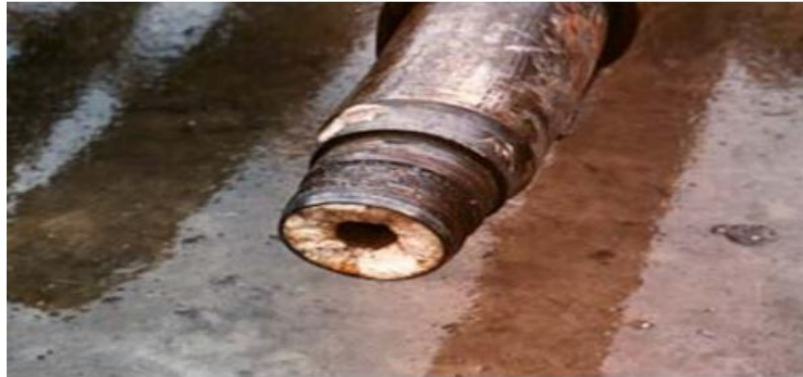
Figure 1: Example of a pipe with mixed BaSO 4 and CaCO 3 Scale from the North Sea. Courtesy E.J. Mackay and K.S. Sorbie. SPE 56775, October 1999.
