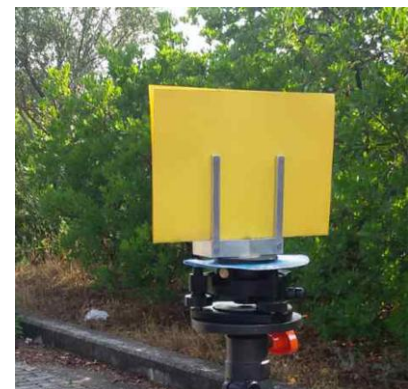
Figure 2. The special supporting base with the goniometer under it and the yellow paperboard on the special supporting base
